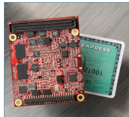
FIGURE 3: A picture of the SFF-COM card showing its size relative to a credit card: This is the bottom side of the board and shows the COMIT 240-pin connector at the top. (Courtesy WinSystems)
