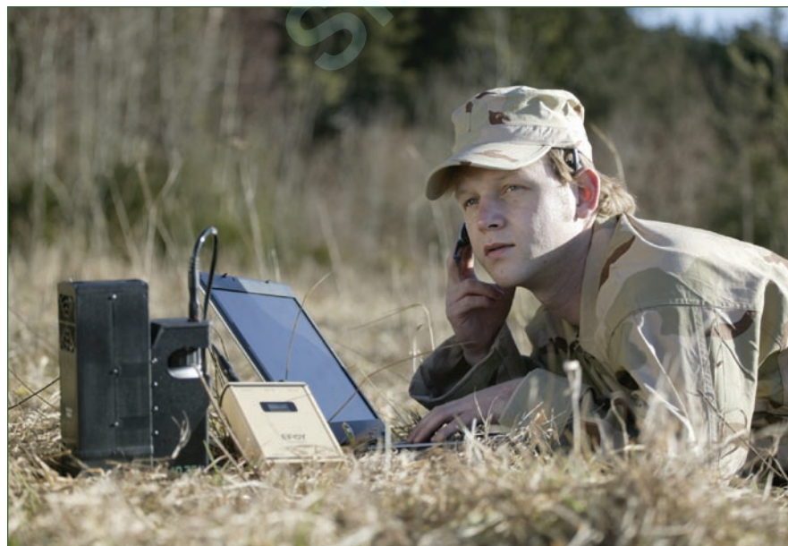
FIGURE 2: The Jenny fuel cell from SFC weighs only 3.7 lbs, plus a 1-lb power manager.
